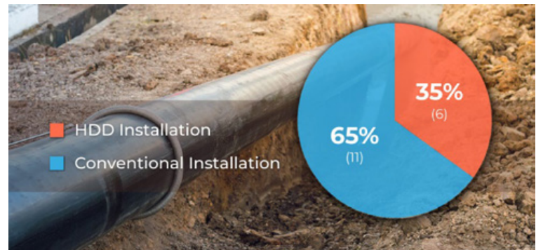
Figure 1. Landslide-pipeline intersections leading to failure by installation type. HDDs are far more vulnerable: out of 162 landslide intersections, HDDs produced 6 failures. By contrast, more than 4,000 intersections with trenched pipe led to only 11 failures
