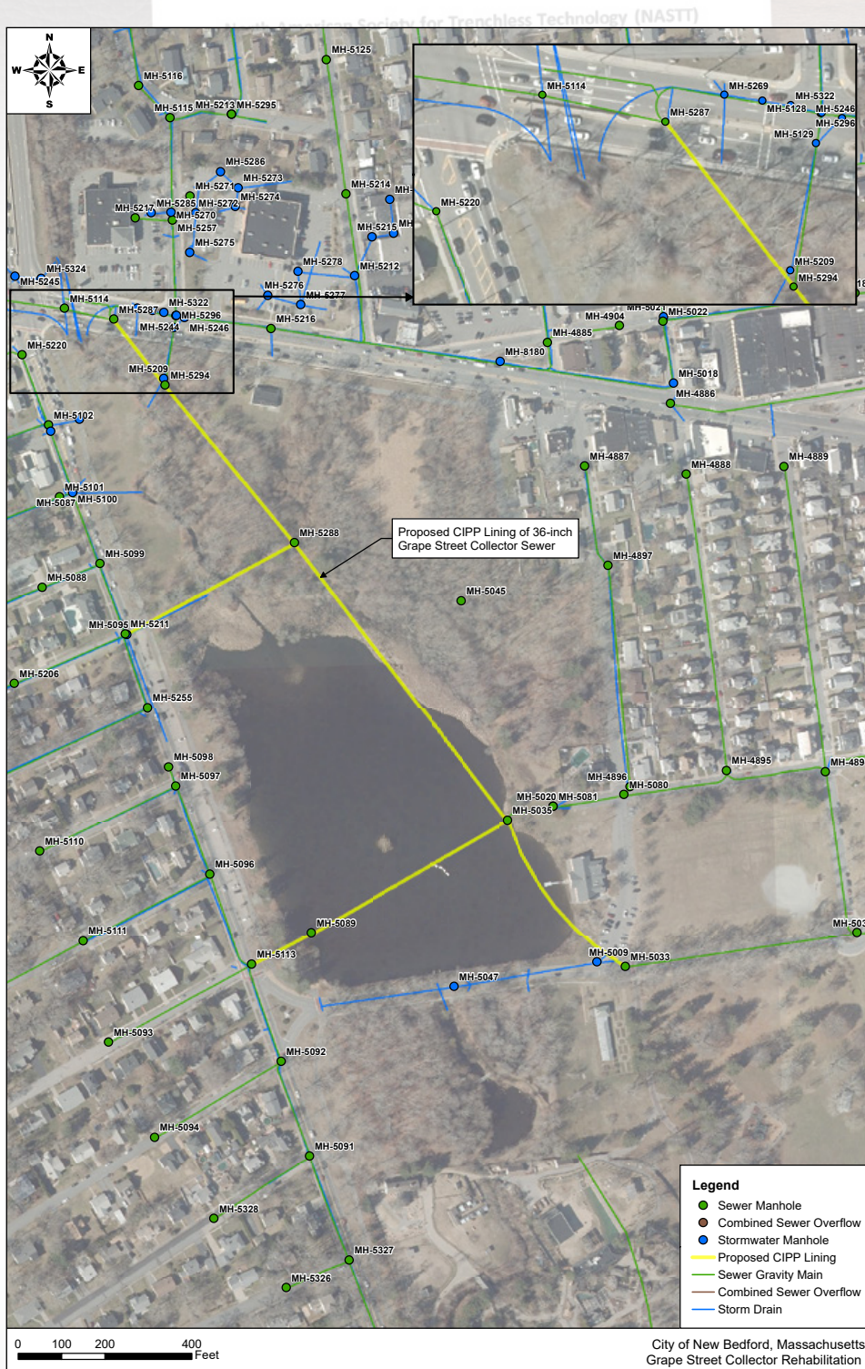
Figure 3: Portion of the Grape Street Collector Sewer Prioritized for Rehabilitation
