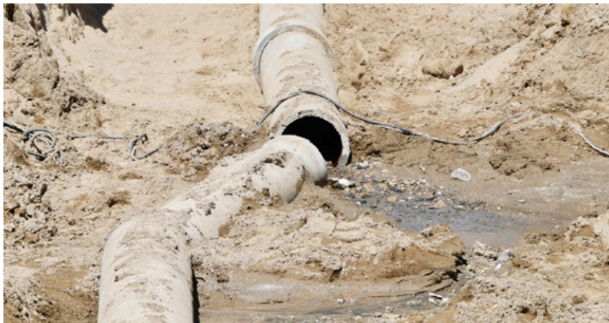
RIDGECREST, Calif. - A formerly straight section of pipe broken by shifting earth during a 7.1 earthquake that shook Southern California in July 2019, cracking buildings, breaking roads and causing power outages. The quake, centered 11 miles from the Ridgecrest area, is the largest quake to hit Southern California in at least 20 years. It was followed by a series of large and small aftershocks, including a handful above magnitude 5.0. (Credit: Gene Blevins/ZUMA Wire/Alamy Live News)
