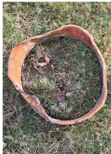
During auger boring at the outset, the casing waffled and the cutting head could barely turn
