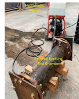
Figure 4. Experimental Setup for External Buckling Testing
