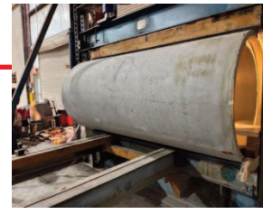
Figure 8. Polymeric-lined Pipe under Three-Edge Bearing Loading Condition
