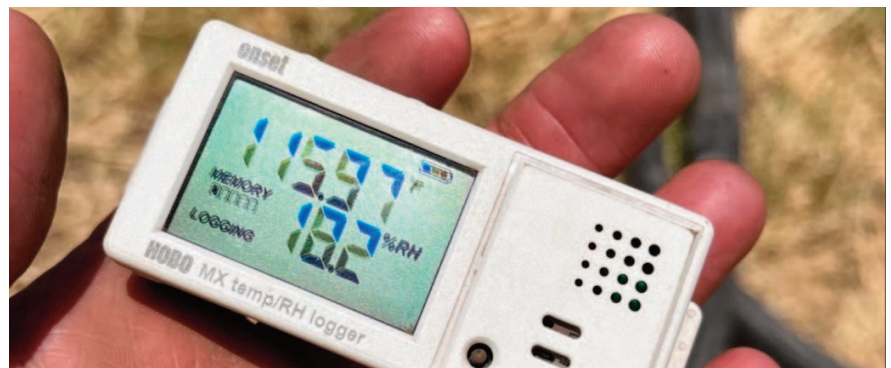
Figure 12. Temperature Reading Inside Pipe (Source: Stephens and Peterie 2025)
