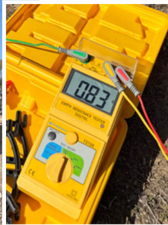
Resistivity measurements were taken as the installation progressed
