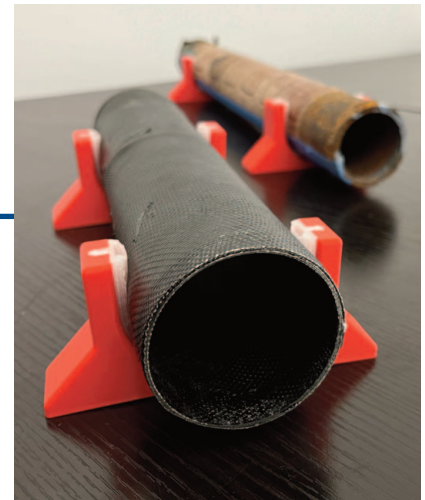
Composite pipe overwrap used for pipeline protection and repair
