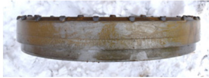
24-inch ring bit - key challenge was accelerated tooling wear from hard and abrasive rock requiring conservative tooling assumptions
