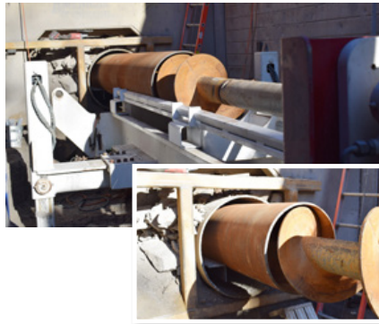
To remain within tooling limits a telescoping approach was implemented
