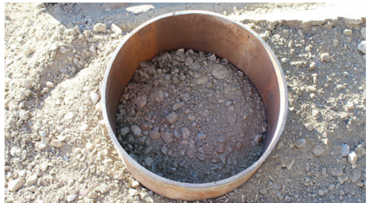
Figure 1. A 24 inch piece of casing is placed over cobbles excavated during preparation of the launch pit (left) The same casing placed over the spoils pile generated by the HHB method during installation (right)
