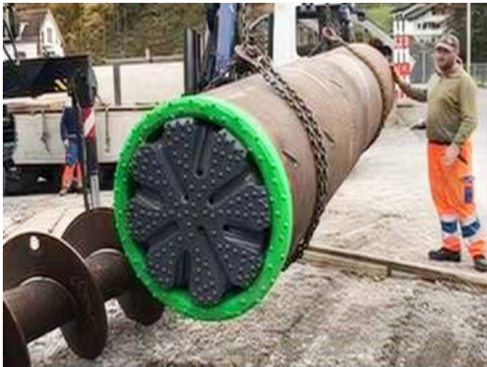
Figure 3. Assembled first section showing ring bit, starter casing and pilot bit
