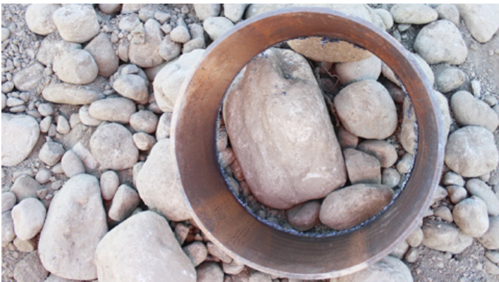
Figure 1. A 24 inch piece of casing is placed over cobbles excavated during preparation of the launch pit (left) The same casing placed over the spoils pile generated by the HHB method during installation (right)
