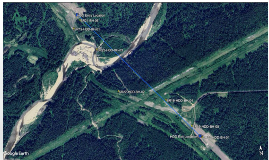
Figure 2. HDD Alignment and Borehole Locations
