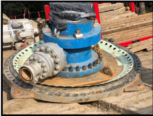
Figure 8 – NPS 72 Rotating Head
